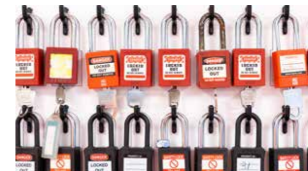
"Always lock-off before you clear blockages, clean, or do maintenance." One of our 10 Lifesaving Rules
