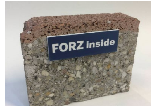
FORZ - Mineralz Making clean building product from bottom ashes of incineration plants
